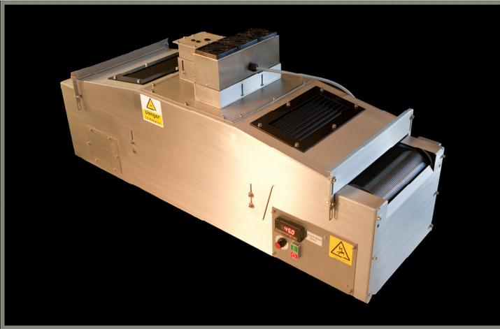
They provide an infinitely variable speed output from a minimum of c.0.2m/min to a max c. 150m/min. The light bridge is height adjustable to allow for differing products flood versus focus testing/applications.
